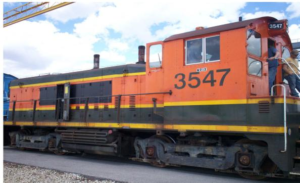
We purchased a new locomotive.... well a new locomotive to us. It's a 1957 vintage EMD (Electro Motive Division of GM) switcher, a model SW1200. This puts it about 10 years newer than our existing locomotive. This should help us to more efficiently load rail.
